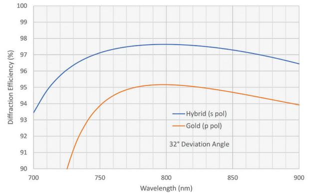
The measured diffraction efficiency of a 195 mm x 55 mm hybrid grating is shown below, demonstrating the high degree of uniformity achievable over the full clear aperture.
